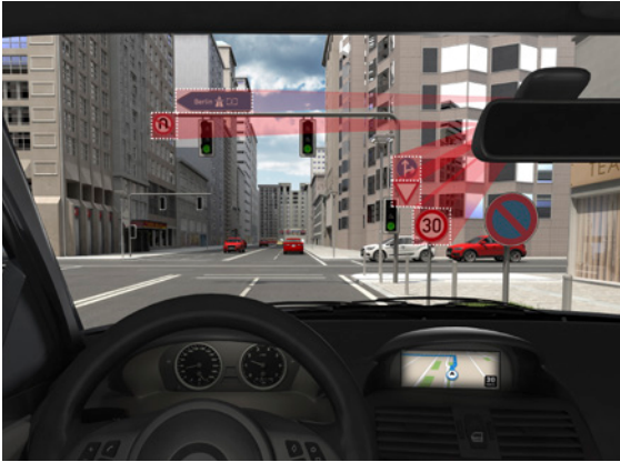
Hella Aglaia Mobile Vision's traffic sign detection system
