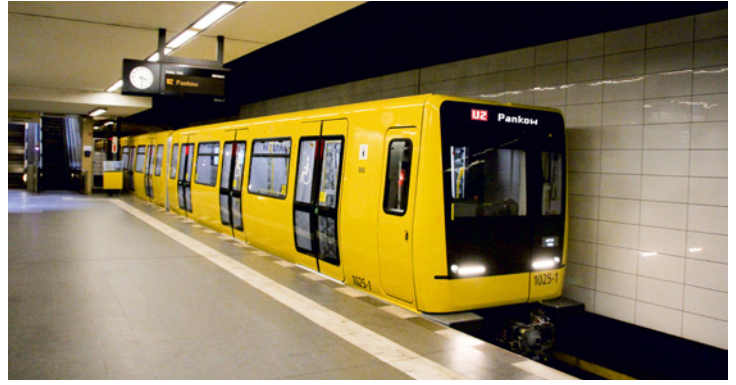
Newly developed underground train for Berlin, called U-Bahn type IK, by Stadler
